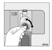
Top up the rinse aid when the indicator light on the control panel illuminates.
